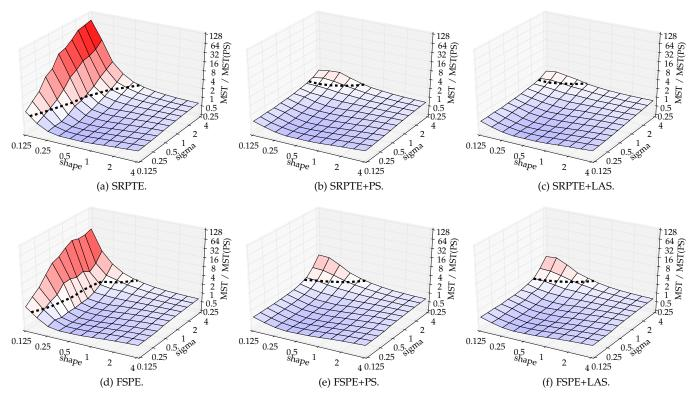
Fig. 3. Mean sojourn time against PS: the dashed line is the boundary where MST is equivalent to that of PS. We recall that a low shape value is associated to high job size skew, while high sigma entails imprecise job size estimates.
