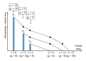
Fig. 2. Example of virtual time t and virtual lag g, used for sorting jobs.
